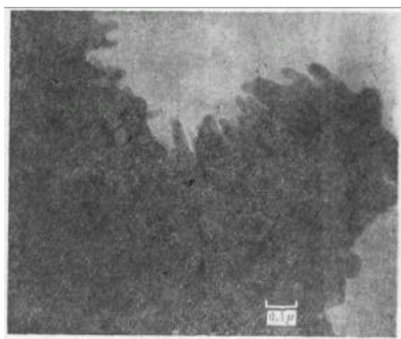
图1 \text{TiCl}_3 (I) 针状晶体, 它们聚集成大颗粒 (71,200 \times )
